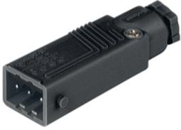
Rectangular Field Attachable Power Connector (ST Series): Male, straight with strain relief , 3-pin+PE, black housing, 400 V AC/230 V DC, 16 A AC/10 A DC
