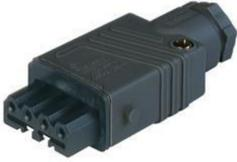
Rectangular Field Attachable Power Connector (ST Series): Female, straight with strain relief , 4-pin+PE, black housing, 400 V AC/230 V DC, 10 A
