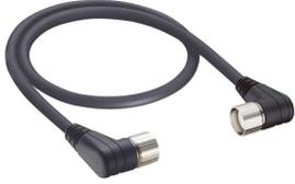
M23 Power Double-Ended Cordset: Male angled to female angled, 12-pin, black body, 120 V AC/DC, 8 A; PUR black cable, 8x0.5 mm<sup>2</sup> + 3x1.0 mm<sup>2</sup>
