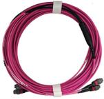
FiberExpress MPO Trunk Assembly, MPO 12 (Male To Male), Multi Mode OM4 (BI), Type B, 2 MPO (24 Fibers), LSZH, 8 Meter, No Pulling Eye, Erika Violet Jacket
