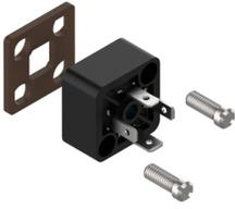
GSSA - Male Receptacle Surface Mount, Form C, Contacts: 3+PE, solder type, 250 V | 6 A, includes EPDM flat gasket; cURus 1977
