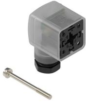
**GDM Standard DIN Standard Field Attachable Connector: Form A, 3-pin (2+1PE; PE across cable outlet), transparent housing, screw type, PG11; with bridge rectifier and yellow LED, 24 V AC/DC, 1 A**
