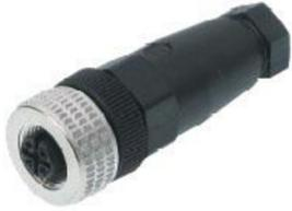
M12 Field Attachable Connector: female, straight, 4-pin, A-coded, unshielded, black housing, screw type, 230 V AC/DC
