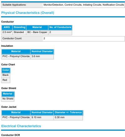
Max. Conductor DCR 8.0 Ohm/km
