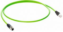
Fast Ethernet Cat5e Data Double-Ended Cordset: Male straight D-coded black M12 Standard to male straight RJ45-coded black RJ45, shielded, 30 V AC / 42 V DC, 1.5 A; PUR green cable, 4-wires, 2x2x0.34 mm<sup>2</sup>
