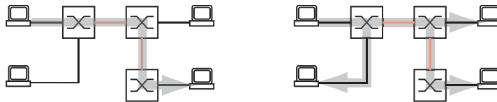
Figure 69: MAC Data Transmission: Unicast Data Packet (left) and Broadcast Data Packet (right)
