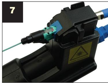
Insert fiber into connector up to the 13 mm buffer mark.
