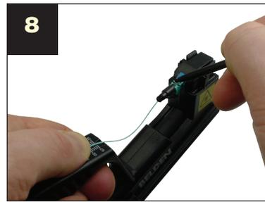
Create and maintain a bow with the fiber, while sliding the activator tab to the closed position (towards boot).
