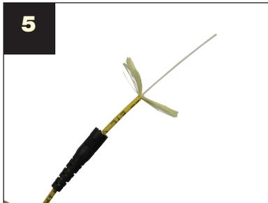
**5** Ensure fiber is fully pushed into jacket, then mark points C, D and E\*
