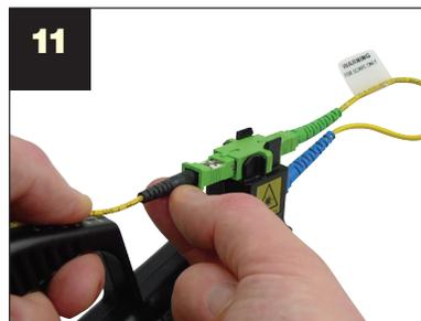
**11** Spread the Kevlar around the threads then gently screw on boot and release bow.
