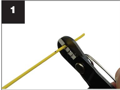
**1** Mark jacket at points A and B, then strip jacket at point A\*
