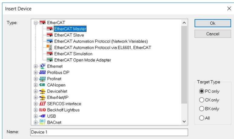
5. If not already done, choose the network adapter and install the driver for EtherCAT® real time communication.
