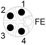
Figure 7: Schematic diagram of the M12 L-coding (connector X03 for Power In)
