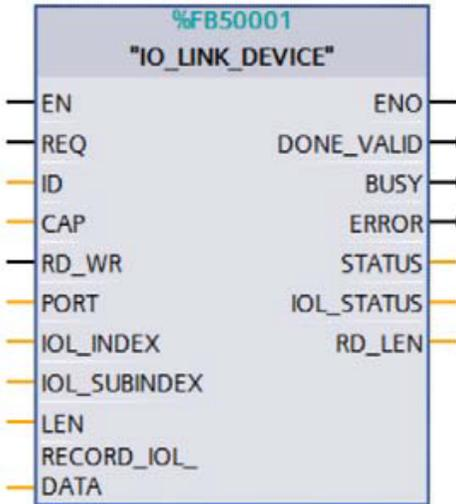
Figure 28: "IO\_LINK\_DEVICE" FB in STEP 7 V15.1
