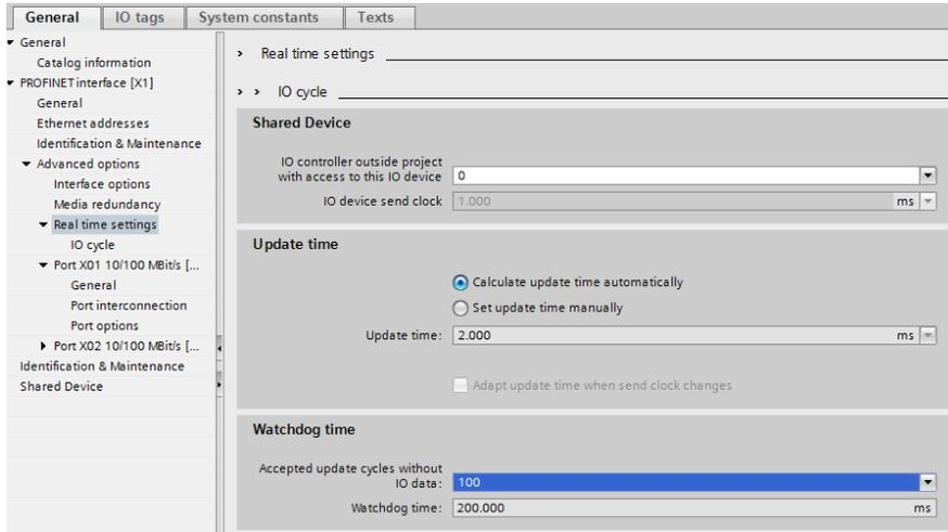
Figure 45: Example of setting up the Watchdog time monitoring in TIA Portal® for using MRP
