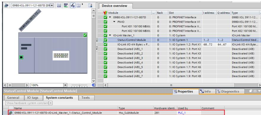
Figure 47: Hardware identifier of the Status/Control Module for RDREC "IO System 1"
