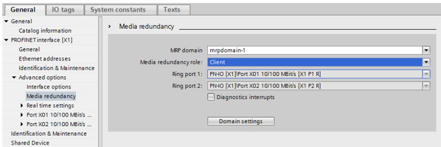
Figure 44: Example of setting up an MRP redundancy client in TIA Portal®
