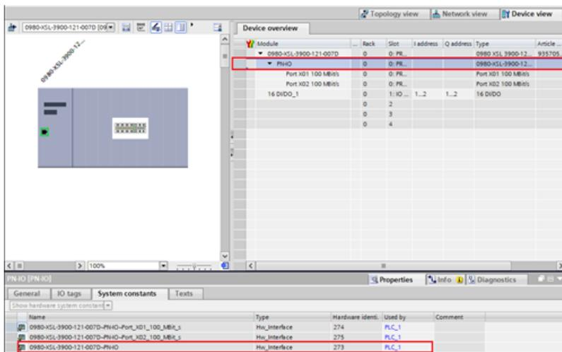
Figure 25: TIA Portal® hardware identifier of PROFINET interface for I&M 0-3 RDREC/WRREC
