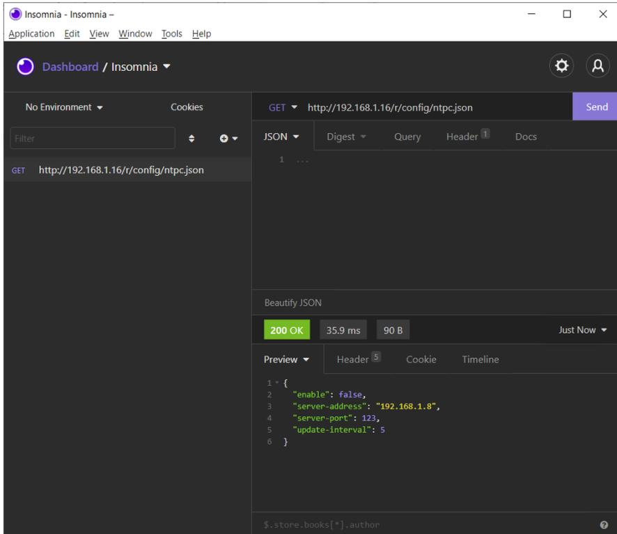
The screenshot shows the Insomnia REST client interface. The top bar displays "Insomnia - Insomnia" and navigation menus. The main area shows a request configuration for "GET http://192.168.1.16/r/config/ntpc.json". The response is displayed in the "Preview" view, showing a 200 OK status, 35.9 ms response time, and 90 B of data. The JSON response is as follows:
