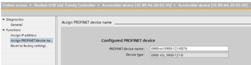
Figure 16: Assign device name
