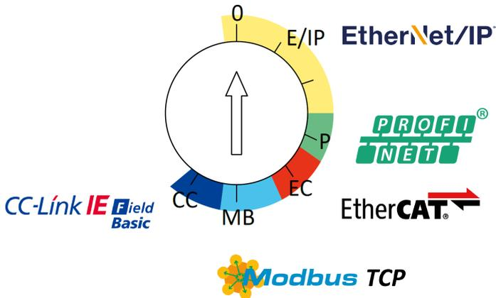
With the other rotary encoding switches (x10 / x1), you set the last two digits of the IP address when you are using EtherNet/IP, Modbus TCP or CC-Link IE Field Basic.
