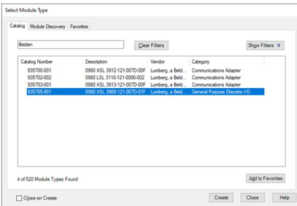
8. Use the **Module Type Vendor Filter** on the right side to display all installed devices of Lumberg Automation™.
