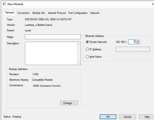
**10.** Enter a name for the device and set the chosen IP address. In this example, the name is **MOD01\_IOL** and the IP address is **192.168.1.1**.
