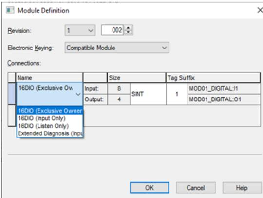
**12.** Select the connection type and configure the total sizes of the input and output process data. The sizes depend on the number of connected devices and their data lengths of both directions. Each device input and output data size must also be set later in the port configuration. The selection of the data type refers to the type in which Studio 5000® maps the input and output data. The default data type is SINT. The INT type is selectable when each size is
