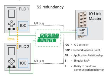
S2 redundancy is a mechanism based on the Profinet signal transmission which allows that the IO-Link Master LioN-P is connected to two different controllers. This enables to transmit sensor & actuator signals from the field level to two redundant Profinet controllers and leads to an increased realiability of applications in e.g. pharmaceutical industry.
