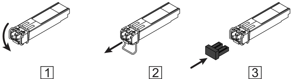
Figure 2: De-installing SFP transceivers: De-installation sequence
