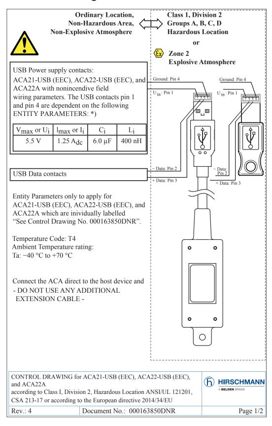
Make sure that the Entity Parameters of the host device meet the following requirements: \*)
