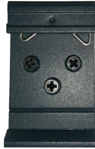
Figure 8: Default position of DIN rail clip
