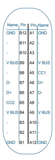
Figure 1: Pin assignment of the USB-C interface
