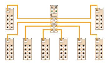
When LioN-Power IO-Link I/O Hubs are combined with the LioN-Power IO-Link Masters, you can **cost-effectively transmit a maximum of 132 digital signals up to 20 m away from the Masters**. It now makes financial and economic sense to upgrade from passive to active systems, or for distributed environments to collect many digital signals.
