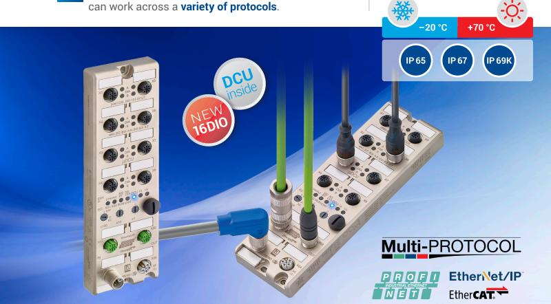
DCUs are IP67 I/O modules with integrated PLC functionality that connect sensors and actuators and can perform simple logical operations of more complex control systems, all without a higher-level PLC. Our modules are now universal with the new 16DIO DCU1. Be certain. Belden.
