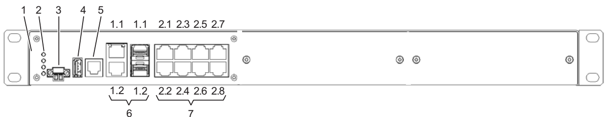
Figure 2: Overview over interfaces, display and operating elements of the MACH102-8TP-F, and MACH102-8TP-FR
