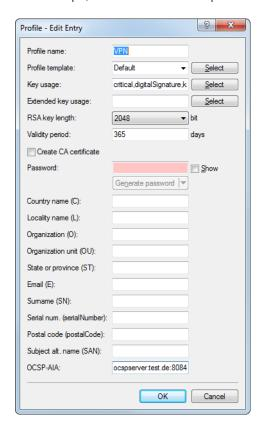
In the example, the default value for the profile "VPN" is adapted to "ocspserver.test.de:8084":
