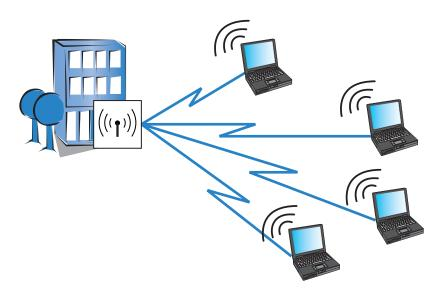
Figure 1: A single access point connected to wireless clients
