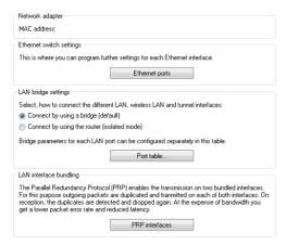
**5.** Enable the PRP interfaces and set the interfaces that the AP uses for bundling.
