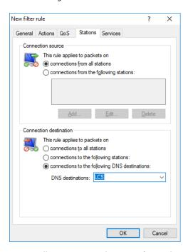
In **Firewall / Qos > IPv6 Rules > IPv6 forwarding rules**you can create a new rule. Entries from the **DNS destinations** or **DNS destination list** tables can be used as **Target stations**.
