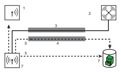
Figure 17: Communication between Access Point and WLAN Controller with CAPWAP tunnel
