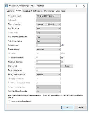
The **Automatic** mode describes the previous behavior, whereas **Manual** allows an absolute value in dBm to be specified in the field **Tx power**.
