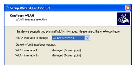
A device can have multiple WLAN interfaces. Here, the selected device has two (2) interfaces. By default, both interfaces are enabled.
