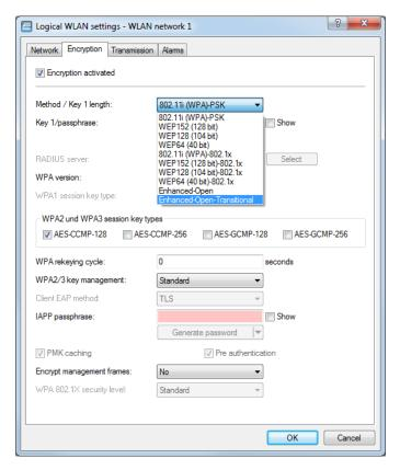
Not only is entering a key not required, it is not even possible: A client enabled for Enhanced Open establishes an encrypted connection to the access point without any key having to be entered. To the user, it is just like using an unencrypted, open WLAN: There is no need to enter any previously communicated key as with WPA2-PSK.
