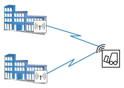
Figure 6: A WLAN client roaming between access points
