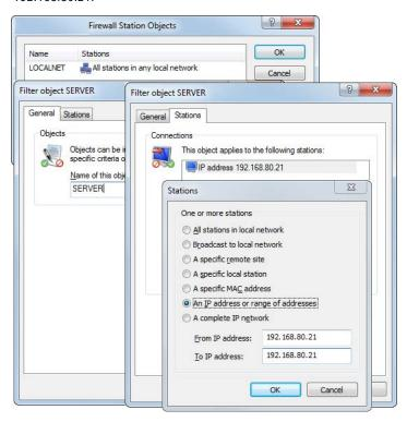
3. Next, go to Firewall/QoS > IPv4 rules > Firewall rules and create a filter rule.
