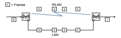
In applications with difficult conditions (moving parts, high temperatures), the wireless link acts as an automatic backup to a wired connection.
