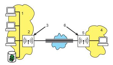
Figure 75: Automatic VPN function with coupled LANs
