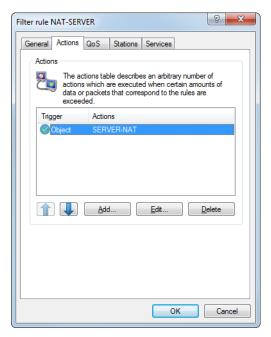
**5.** Then go to **Stations** and use the newly created station object. If necessary, you can also specify the Internet line under **Connection destination**.
