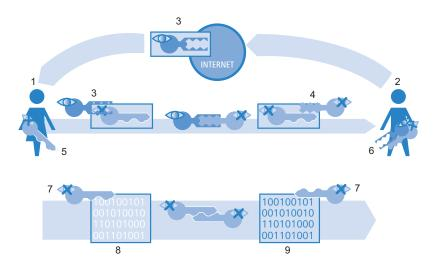
Figure 81: Combination of symmetrical and asymmetrical encryption
