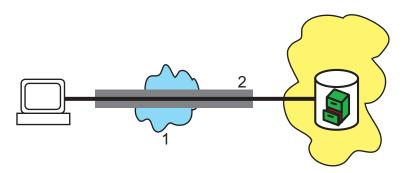
Figure 69: VPN data transmission in IPSec transport mode
