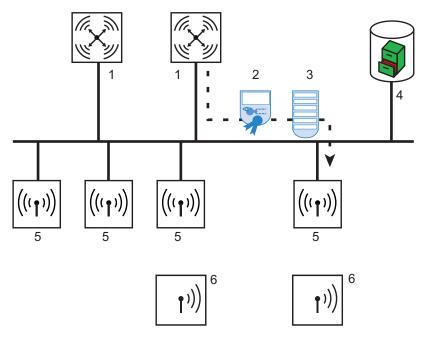
Figure 11: Configuring several Access Points with one WLAN Controller
