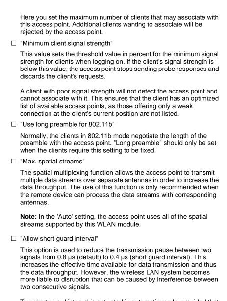
The short guard interval is activated in automatic mode, provided that the remote station supports this. Alternatively the short guard mode can be switched off.
