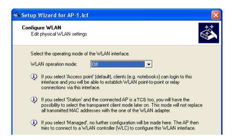
A point-to-point WLAN bridge requires just a single interface. In this example, the currently selected interface—WLAN interface 2—will be disabled. (You will later configure WLAN interface 1 to support the point-to-point WLAN bridge.)
