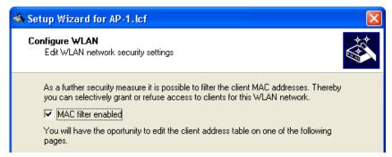
The OpenBAT device can filter WLAN Client devices based on a list of MAC addresses. The list can be either a:
