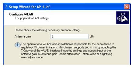
the calculated antenna gain is 8 dBi for this example
