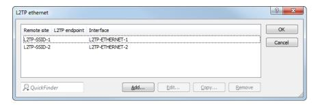
In our scenario, the payload data of all connected access points are routed to the virtual interface configured here. Furthermore, the payload data of all access points connected to this virtual interface are bridged to one another—rather like the WLAN controller-based layer-3 tunneling technique.
