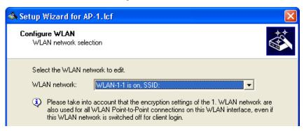
For the WLAN network, select 'WLAN-1-1'. This indicates that this access point will use channel 1 on interface 1.
