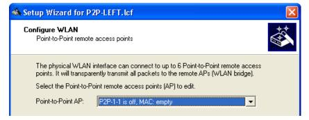
Each OpenBAT device supports up to 6 point-to-point channels. Select an available point-to-point channel for this WLAN interface.
