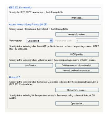
The device offers the ability to individually enable or disable and configure the support the IEEE 802.11u standard as well as the Hotspot 2.0 functionality for each logical WLAN interface using the button "Interfaces".
