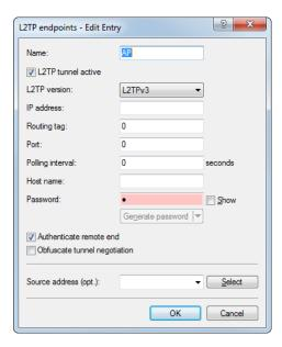
The **IP** address is empty. This is then a "wildcard" entry that can accept connections from any remote site.
