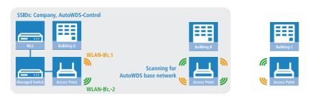
Figure 4: Phase 1 – unassociated AP in building B seeks AutoWDS base network and finds anchor AP in building A
