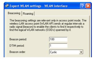
Configure the beaconing settings to influence the transmission of beacons by the OpenBAT device in its role as Access Point. These settings can influence the roaming behavior of clients, and optimize Multi-SSID operations for older WLAN Clients.
