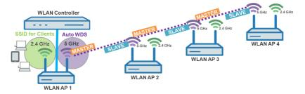
Figure 9: Connection lock after DFS detection
