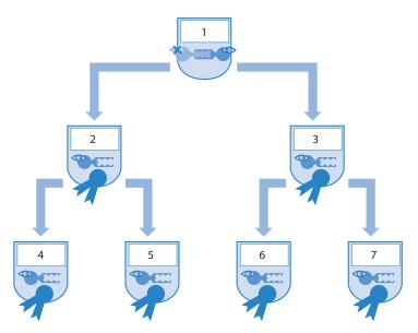
Figure 105:Multilevel certificates for SSL/TLS
