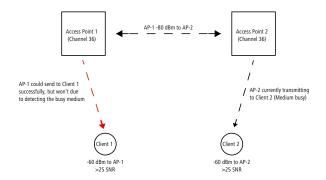
An access point can be set artificially "deaf" by reducing the reception sensitivity from HiLCOS 10.32 onwards. This means that transmissions further away from the access point are "overheard" and the channel is detected more often as "free". In simplified terms, more simultaneous transmissions on the same channel are possible. On the one hand, this increases the overall throughput of a system, but on the other hand, the interference on the client side also increases.
