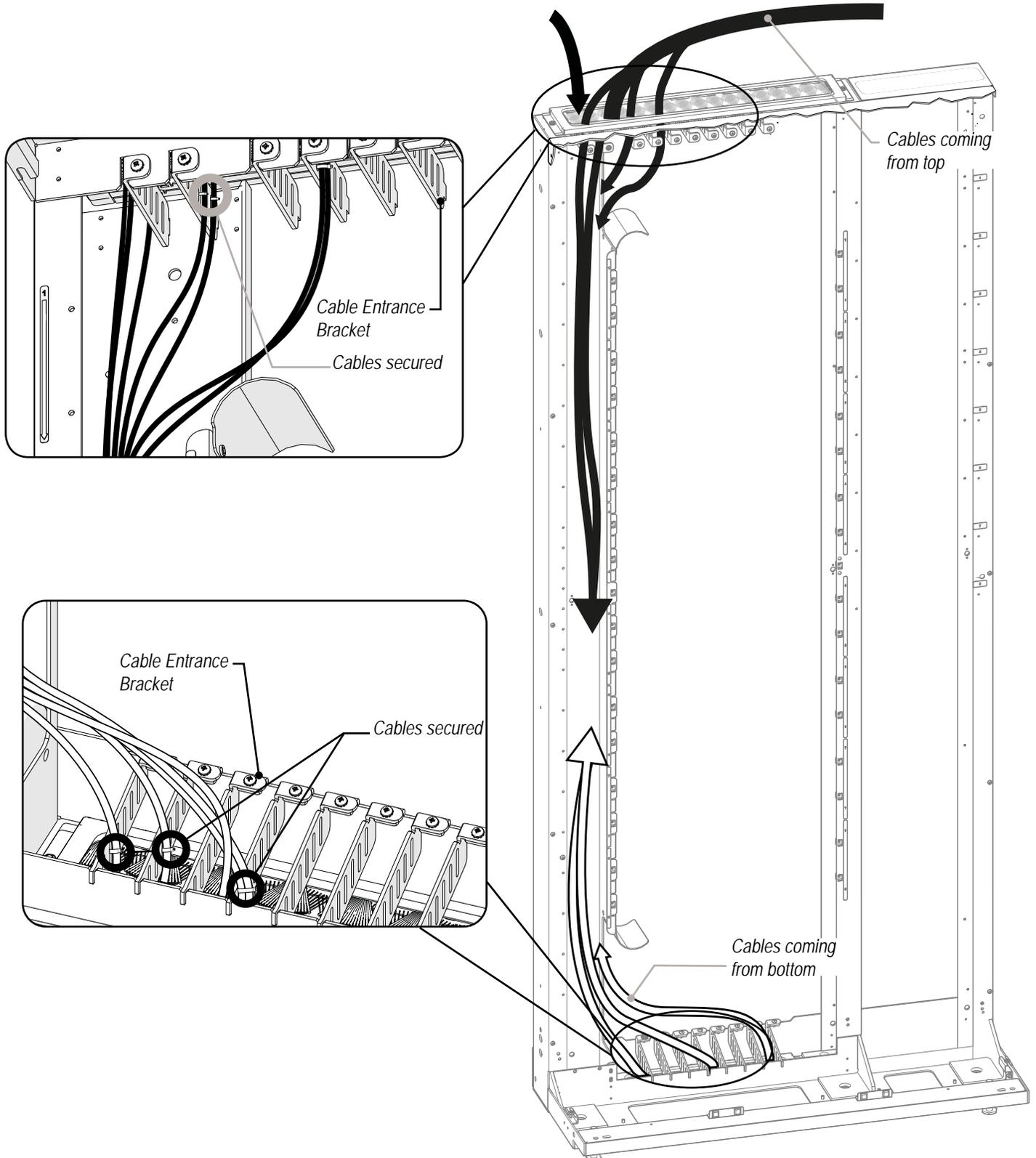
2. Install the Housing into the Cabinet and use the visual reference to determine the Cable Distribution Bracket position. Once the position is determined, install the Cable Distribution Bracket on the Cabinet by using the provided screws.
