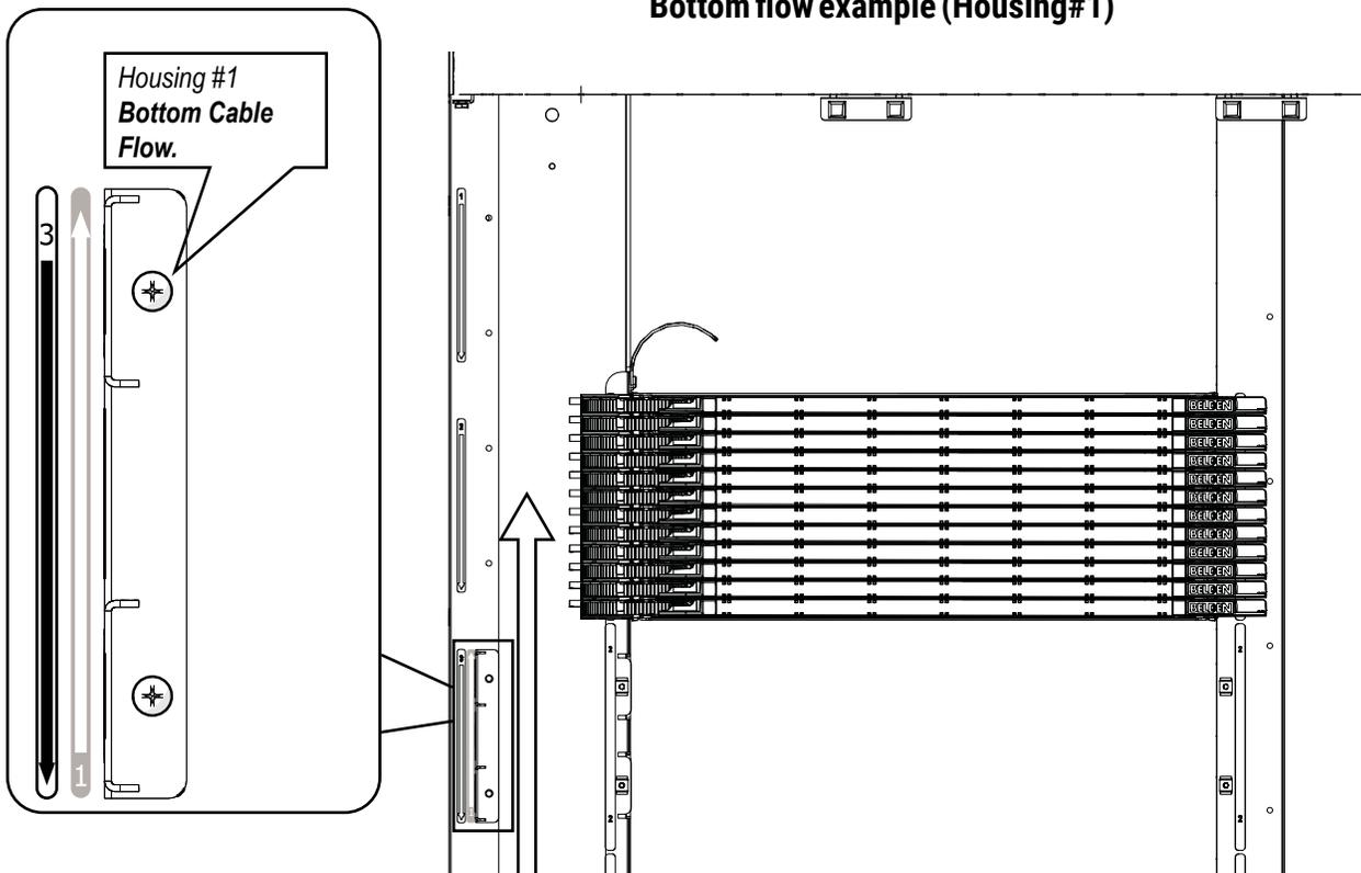
**3. Determine the angle of the Cable Distribution Manager based on the cable flow.**
