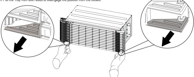
2. To open the Tray completely, squeeze the front latch and pull both sides of the tray.
