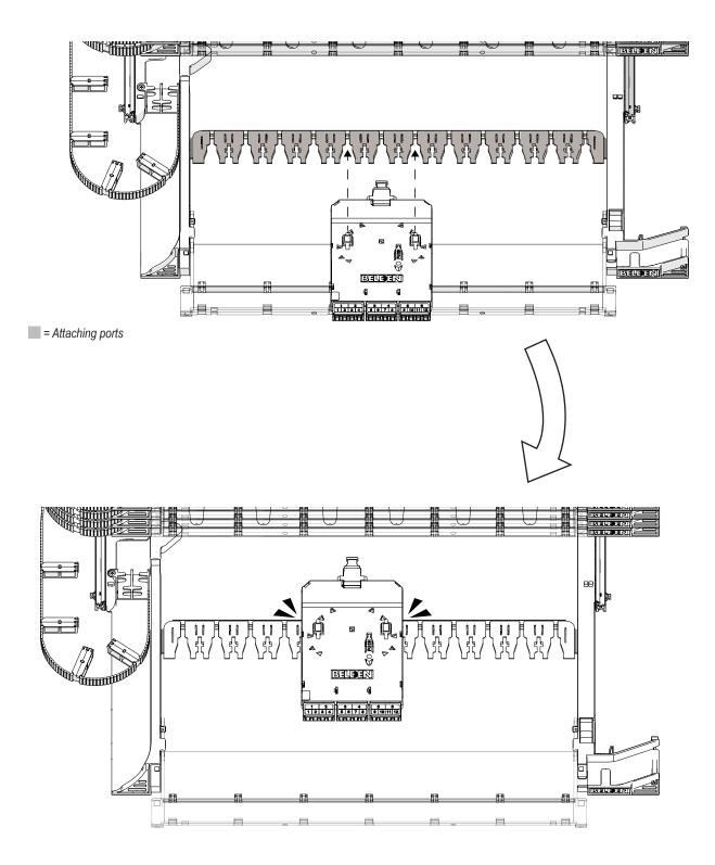
**3.** To remove the Cassette/Adapter Frame from the Tray, press on the latch and slide the component outward.
