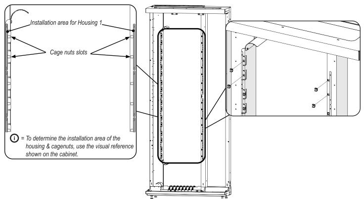
Once the installation area is determined, align the Housing brackets to the installed cagenuts. Use the provided screws to secure the bottom (or top) of the brackets. Repeat the previous procedure to secure the remaining sides of the brackets.
