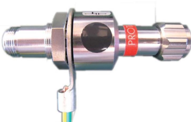
Figure 7: Grounding the BAT-ANT-Protector m-f
