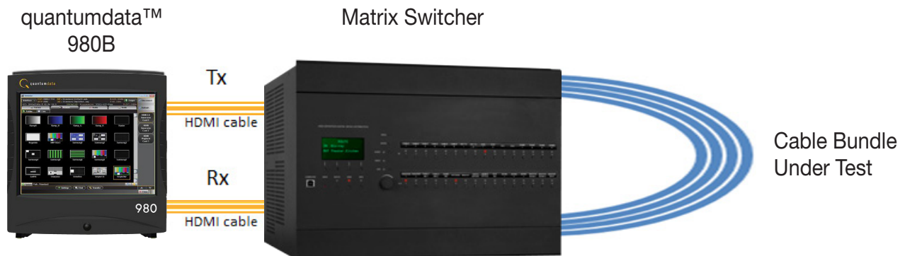
Figure 7: Test Set-Up to Measure External Noise Effects on Transfer Quality
