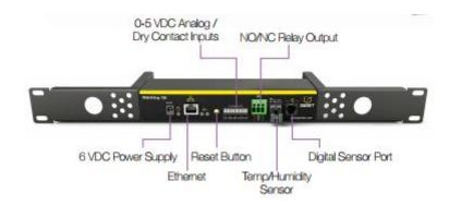
The Watchdog 100 is a self-contained unit with an on-board temperature/humidity/ dew point sensor. It has an input capacity of eight external sensors and relay output for triggering external devices, such as an auto-dialer. Built-in Power Over Ethernet.
